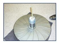
This supporting rod is then held firmly and aligned by the top and bottom of the central spigot.
