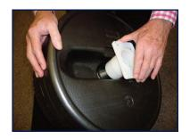
The central spigot is then screwed into the white base so that the whole assembly is held tightly on to the base.
